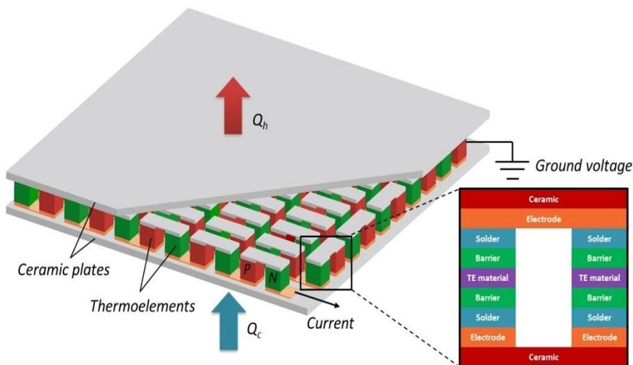
Fig. 2 Constructional cross-sectional view of TEC module
