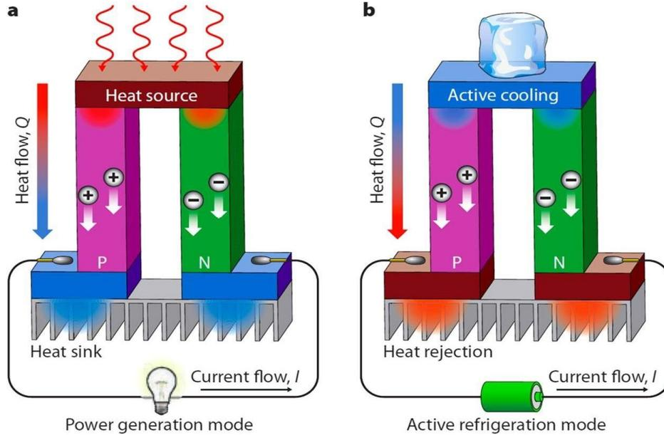
Fig. 4 Working principle of seebeck and peltier effect
