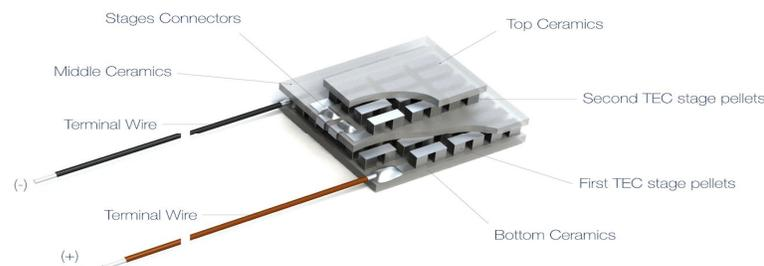
In multi-stage TECs every previous stage cools down the next one. Thus the resulting  $\Delta T$  between hot and cold sides is higher comparing to a single-stage TEC. TECs with 2, 3 or 4-stage solutions are common, in some rare cases - 5 or 6
