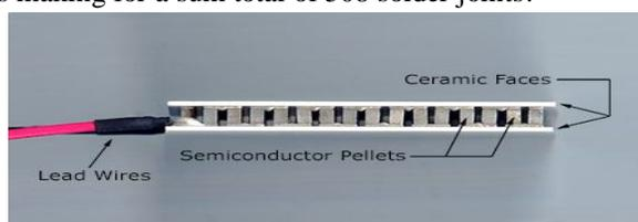
Fig. 8 Side view of an unsealed TEC module
