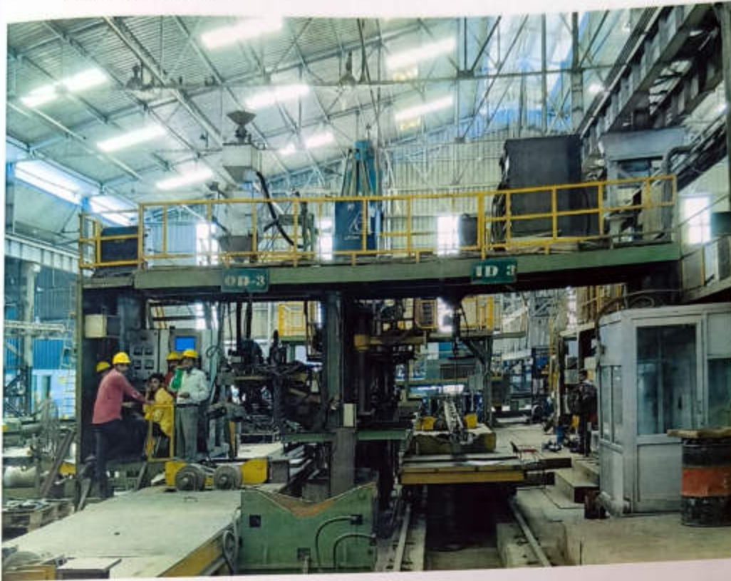
fig.4.7 ID OD SAW Welding courtesy of Jindal
