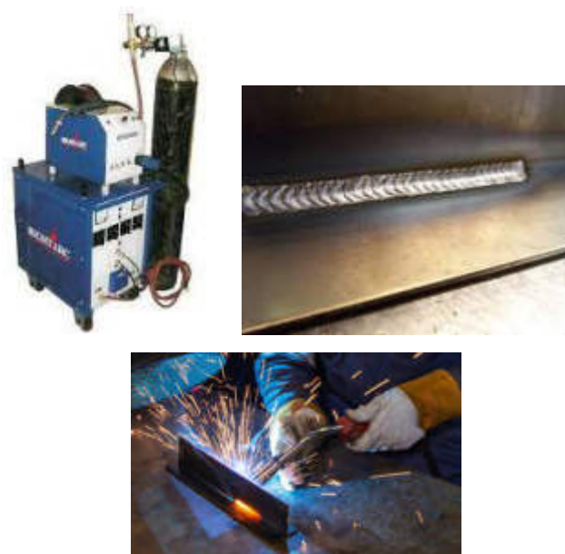
Fig: 2.30 Mig Welding Process and Machine
