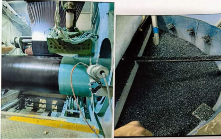
fig.5.5 PP/PE Coating courtesy of Jindal
