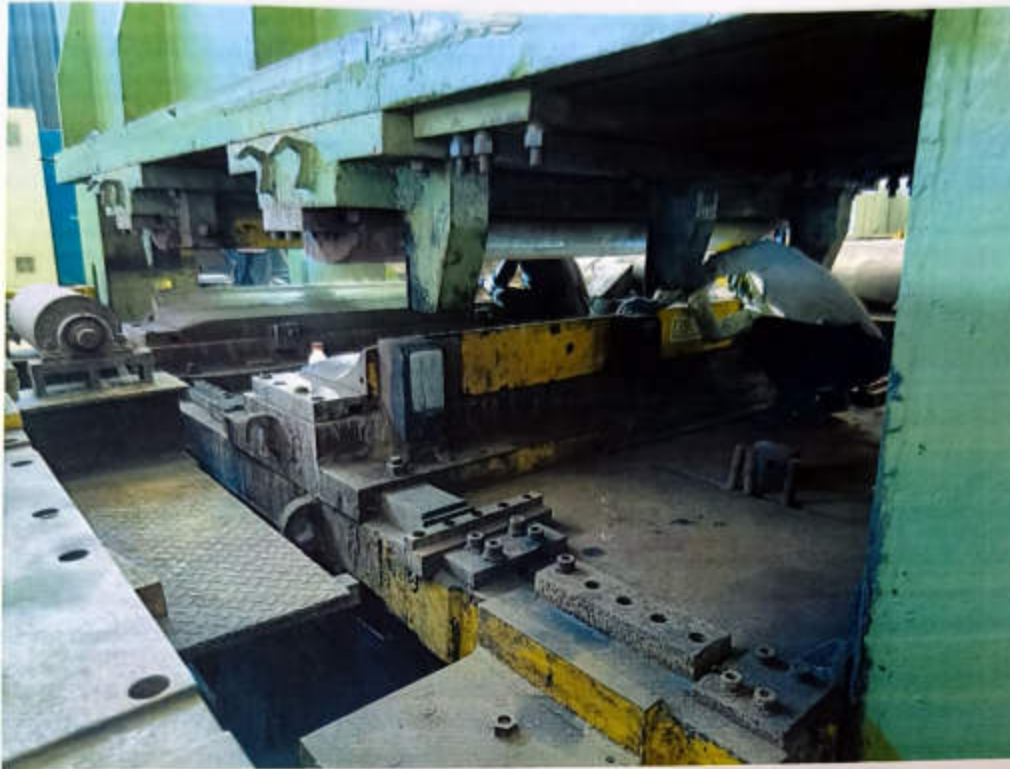
fig.4.4 Pre Bending Machine Courtesy of Jindal
